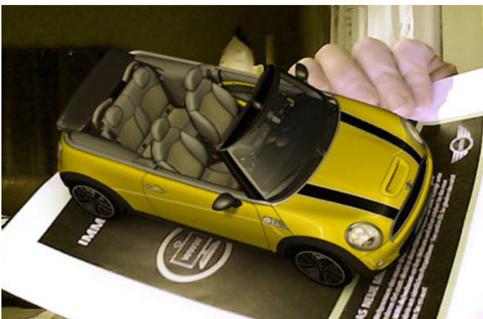
Fig. 5: An advertising campaign for the automotive company MINI, where the user holds the ad in front of a webcam and sees an animated 3D MINI 'pop-up' on the page.
